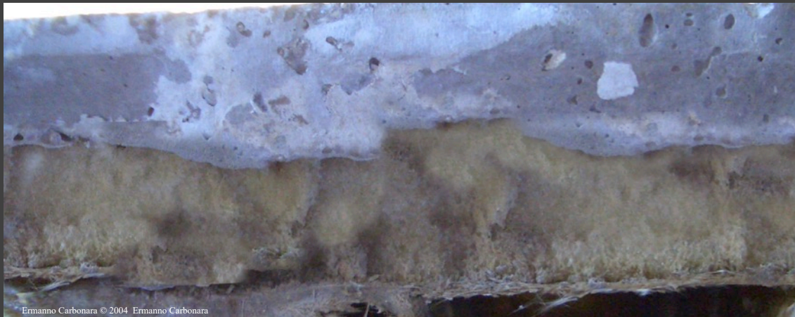
Panel made up of polyurethane foam between two layers of resin reinforced with fiberglass
