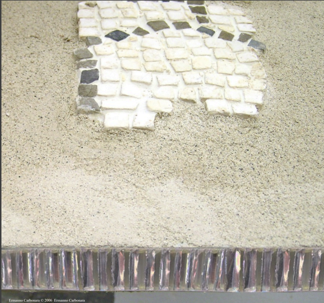
Panel made up of aluminum honeycomb between two layers of resin reinforced with fiberglass
