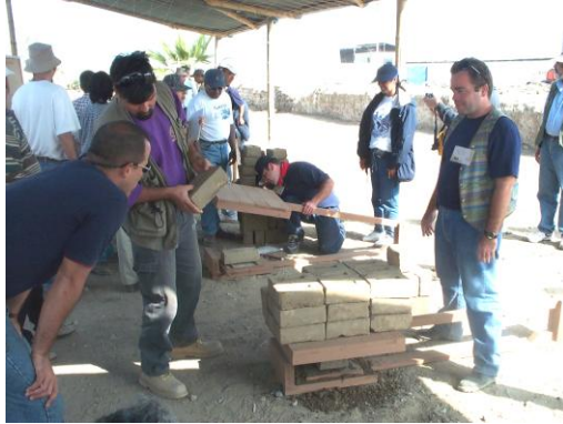
Figure 3.3.5 (left) and 3.3.6 (right) Students performing flexural strength in-situ test (left) and discussions about the performance of the different molds (right) PAT course, 1999 © J. Paul Getty Trust
