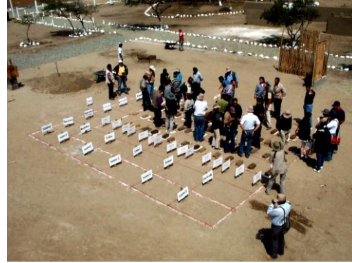
Figure 3.3.5 (left) and 3.3.6 (right) Students performing flexural strength in-situ test (left) and discussions about the performance of the different molds (right) PAT course, 1999 © J. Paul Getty Trust
