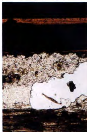
Figure 2. Fifteenth century, heavy black layer. A new photograph of a thin-section from Garner's estate in transmitted light (16x). From bottom to top: wooden base; heavy black layer (mostly broken away); very thin transparent lacquer layer (looks orange); dark, yellow ground layers; black guide line (Garner 1963) looks transparent orange (see text); red ornamental zone. Figure 3. Thin section of a Han dynasty lacquerware object from Garner's estate.
