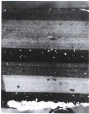
Figure 1. Photomicrograph of a cross section from a Chinese lacquerware object, late sixteenth century, from the estate of Sir Harry Garner (Victoria and Albert Museum, London), taken by A.R. Sollars, Cranfield (magnification x50), supplied with the following commentary on the layer construction: "band 1: 2 layers brownish-red, moderately fine with large inclusions; band 2: 5 layers light red, fine; band 3: 4 layers bright red, coarse; band 4: 1 interface layer, discontinuous, fine layer, grayish; band 5: 1 layer dark gray or black, structureless compared with normal pigmented layers; band 6: 3 brownish-red, similar to band 1; band 7: light red, fine, similar to band 2; and band 8: bright red, coarse as band 3."
