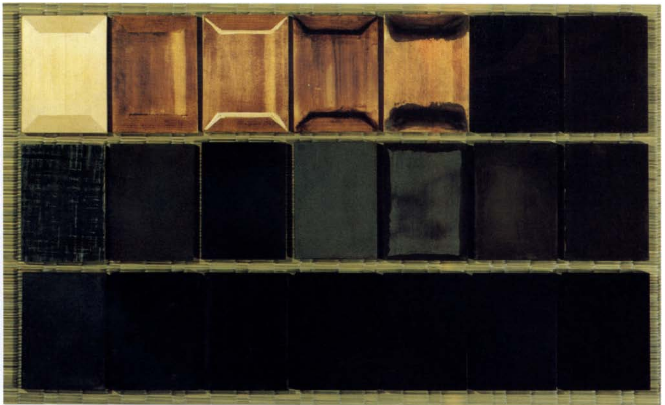
Figure 2. Sample boards showing steps in the process of lacquering, from the basic shape (top left) to the finished product (bottom right).
