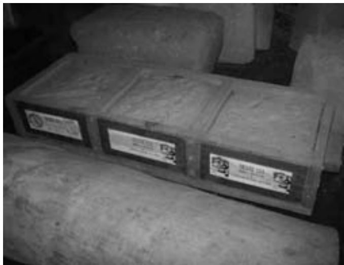
FIGURE 6 Adobe samples amended with hydrated lime and saliva de cupim. Photo: © Honório Nicholls Pereira
