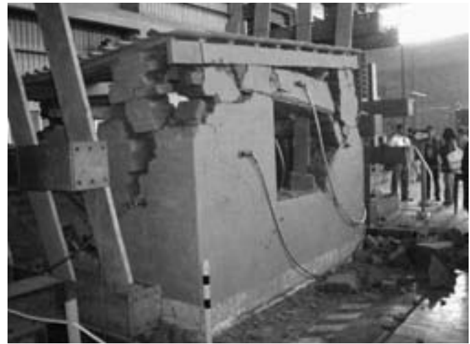
FIGURE 1 Seismic retrofitting tests performed during SismoAdobe 2005, held at PUCP, Lima, Peru, in May 2005. Photo: Mariana Correia
