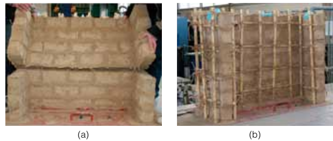
FIGURE 8 Failure pattern of (a) model L-3 and (b) model L-4.
