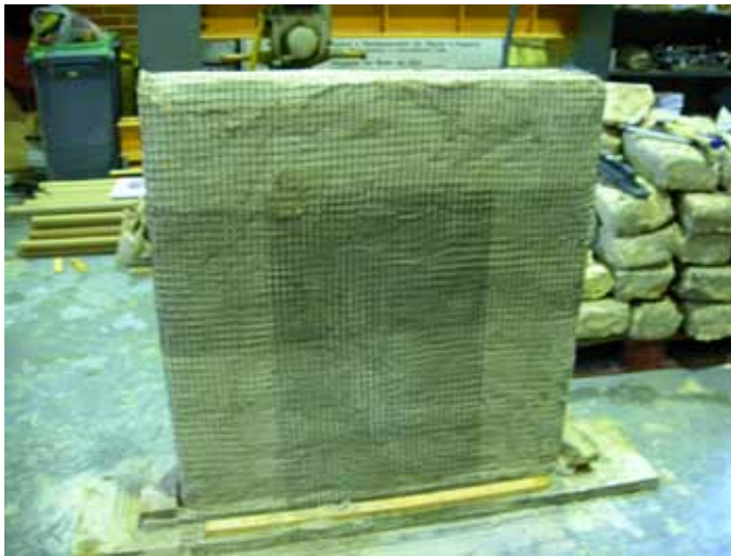
FIGURE 8 Strengthening of an adobe wall with a polymeric mesh and a coat of traditional earthen plaster. Photo: Pereira, 2008
