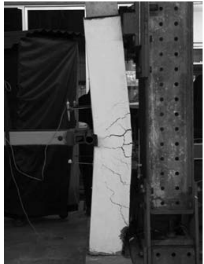
FIGURE 7 Wall tested in flexure out of plane, last phase. Photo: Daniel Torrealva
