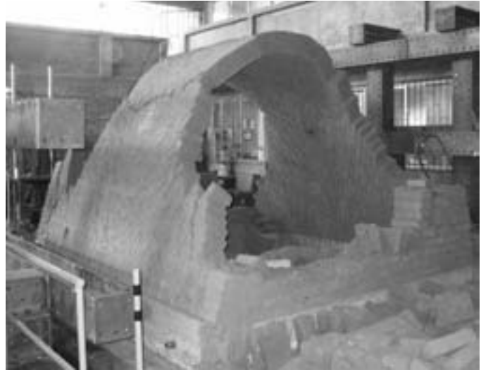
FIGURE 4 Nubian vault without reinforcement of geo-grid and without mud stucco after seismic simulation test.
