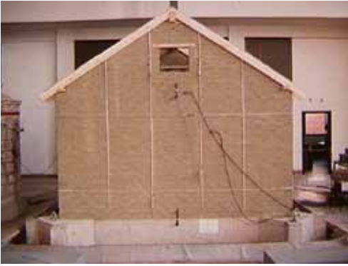
FIGURE 2 Large-scale model building tested as part of the GSAP research program. From Tolles et al. 2000
