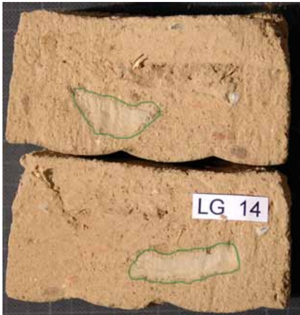
FIGURE 6 Grout behavior in the cavities.
