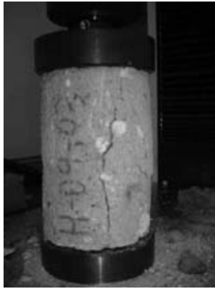
FIGURE 2 Compression testing of an adobe specimen. Photo: Pereira, 2008
