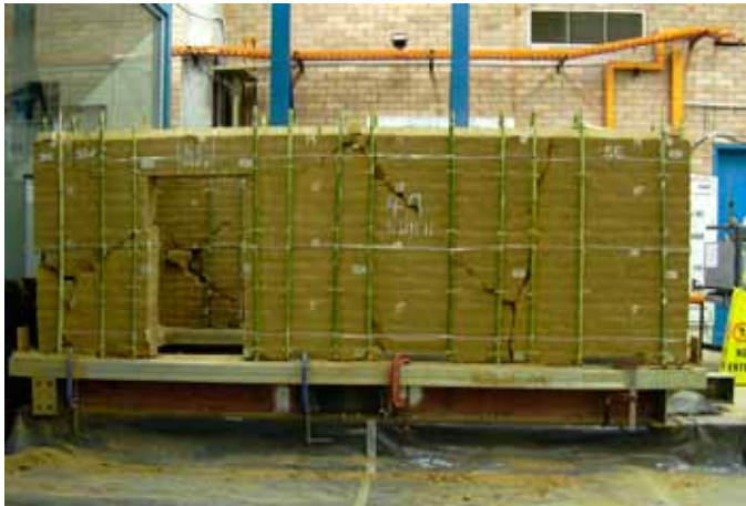
FIGURE 7 1:2 scale adobe house, damaged but intact after a series of severe shake table tests. Courtesy of University of Technology, Sydney, Australia, 2005
