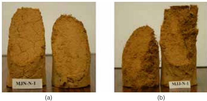
FIGURE 6 Photographs showing failure pattern of sandwich specimens prepared with (a) unreinforced and (b) jute-reinforced mortar.
