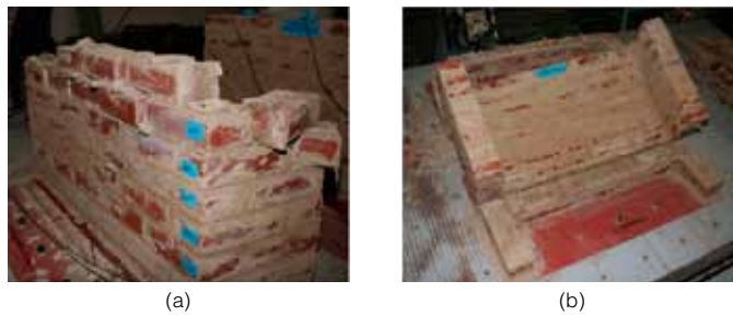
FIGURE 7 Failure pattern of (a) model L-1 and (b) model L-2.
