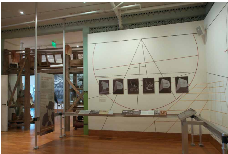
Figure 3 The exhibit system is made up of vertical two-inch-diameter floor-to-ceiling support poles that distribute data and electrical from the floor into the system. Horizontal satin-finished aluminum I-beam members provide a wiring chase and support reader-rail graphics touchscreens and media equipment boxes. Photo: IQ Magic
