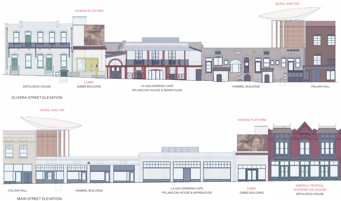
Figure 3 Street elevations of the proposed mural shelter and viewing platform in the context of the buildings included within the project scope. Drawings: Brooks + Scarpa
