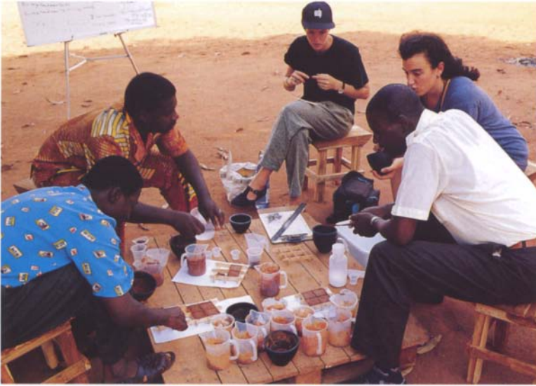
The conservation team making mortar mixes and test blocks.
