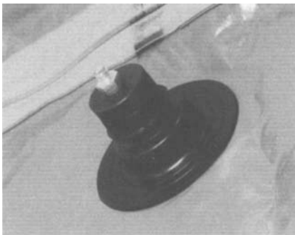
Figure 5.20 An O-ring connector is installed on a Portable Bubble port to be used as a nitrogen inlet or outlet.
