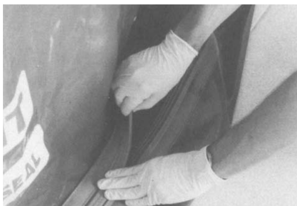
Figure 5.22 Closing the lightly greased zip-lock that holds the Portable Bubble top to its base
