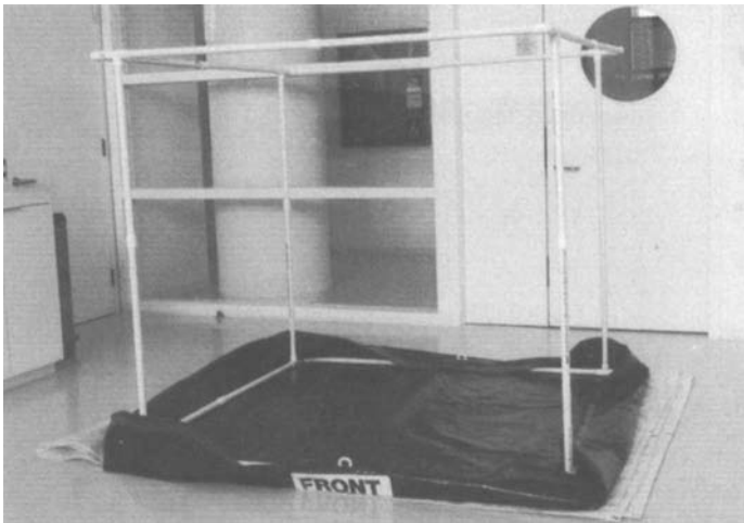
Figure 5.19 Supportive frame for the 6 m 3 Portable Bubble, made from PVC tubing and fittings
