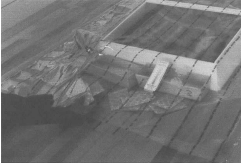
Figure 3.3 Oxygen absorber packets and humidity buffering material (RH-adjusted silica gel) are placed in the bag after most of the heat seals have been completed.
