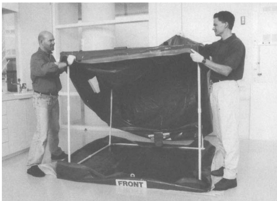
Figure 5.21 The Portable Bubble top is placed over its supportive frame.
