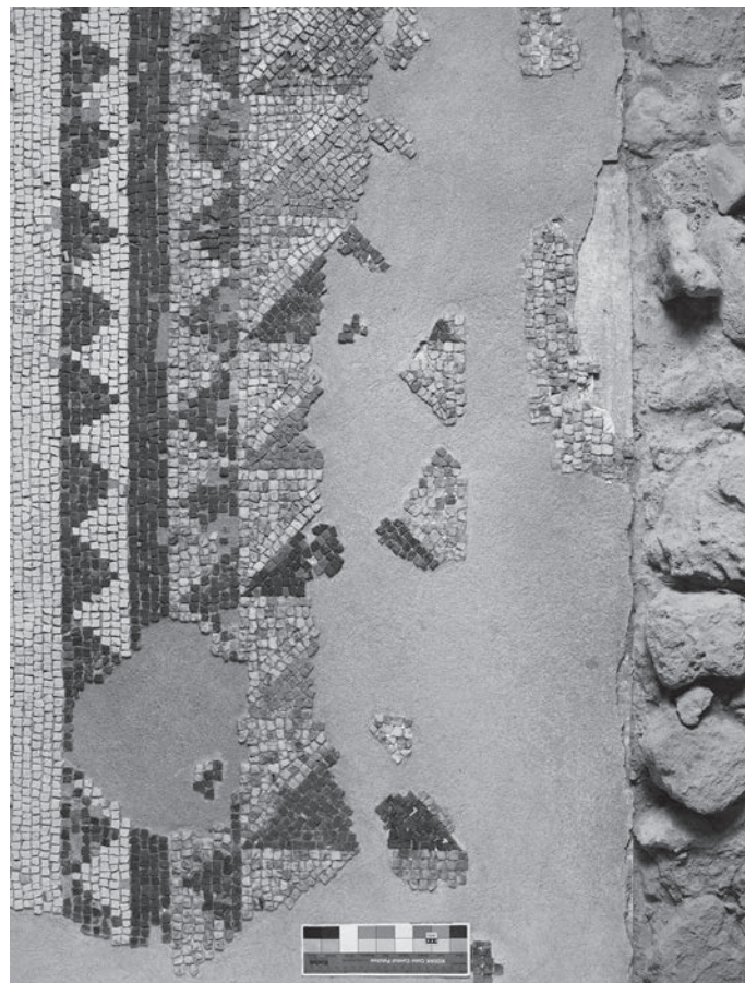
FIGURE 5 Loss of tesserae that had been embedded in polyester resin soon after the re-laying; loss of infill mortar is visible on the right. Photo by Vassos Stylianou 2004. © J. Paul Getty Trust.
