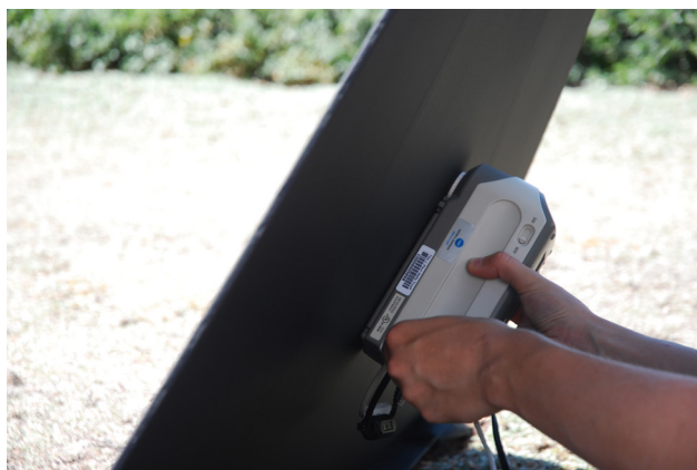
Fig. 5. Handheld spectrophotometer used here for on-site color measurements on an outdoor painted sculpture.
