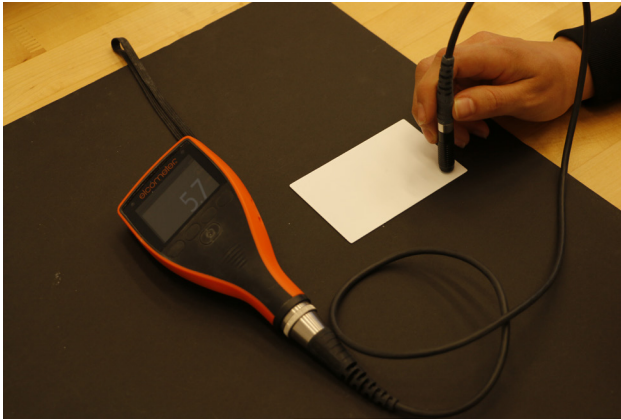
Fig. 7. Ultrasonic thickness gauge applied to measure the paint DFT of a coating after curing.
