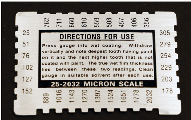
Fig. 8. Notched gauge or comb used to measure the WFT during paint application.
