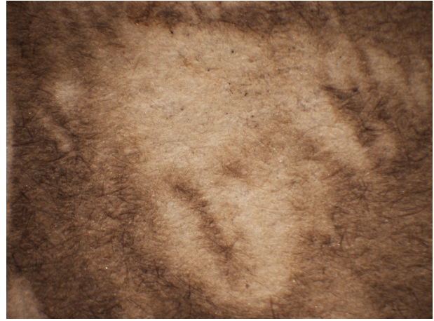
Figure 6b Optical micrograph of a salt print photograph (25x magnification).
