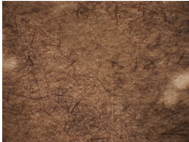
Figure 6a Optical micrograph of a salt print photograph (10x magnification).
