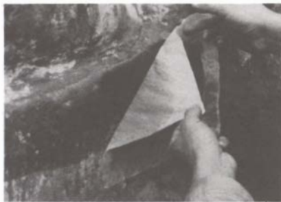
Figure 4. Detachment of the paper without any loss of surface material.
