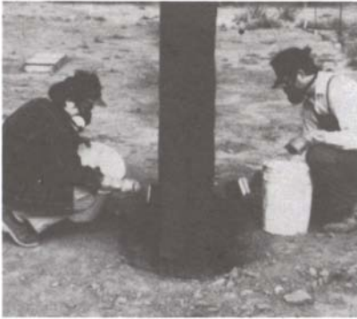
Figure 5. Photograph showing chemical consolidant being brushed onto adobe test wall.
