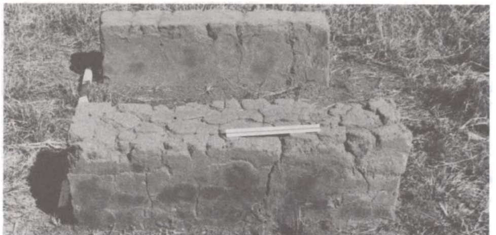
Fig. 5: Experimental wall-after a year of exposure to elements of nature.
