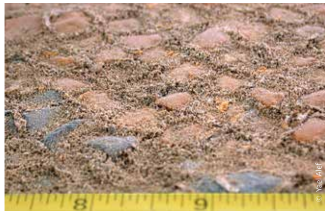
FIGURE 5: The experimental panel (left) shows the severe disintegration of the tesserae caused by the aggressive environmental conditions beneath the experimental shelter over Mosaic NN4, namely relatively high humidity, condensation and accumulation of dust and aerosol on the surface of the mosaic. These phenomena are also evident in the disintegration of the mortar (above).
