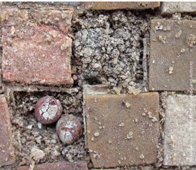
FIGURE 5: The experimental panel (left) shows the severe disintegration of the tesserae caused by the aggressive environmental conditions beneath the experimental shelter over Mosaic NN4, namely relatively high humidity, condensation and accumulation of dust and aerosol on the surface of the mosaic. These phenomena are also evident in the disintegration of the mortar (above).
