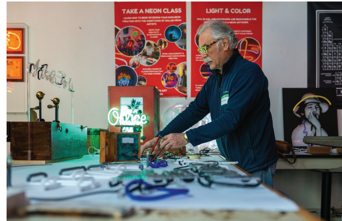
Neon fabricator and artist Michael Flechtner tests a transformer, used to deliver the high voltage needed to make neon glow.
